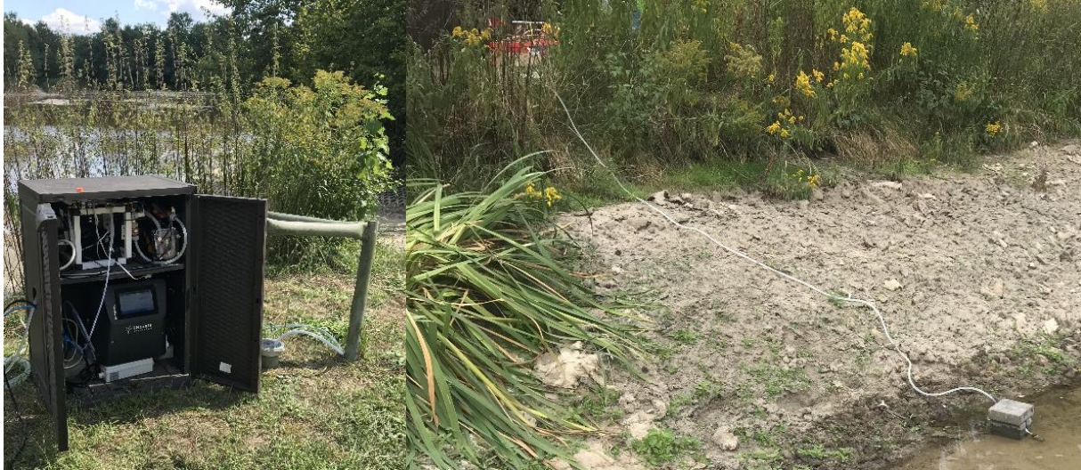
Figure 4: Box with sampling line next to the observation well (left) and intake device at the recharge basin (right).
