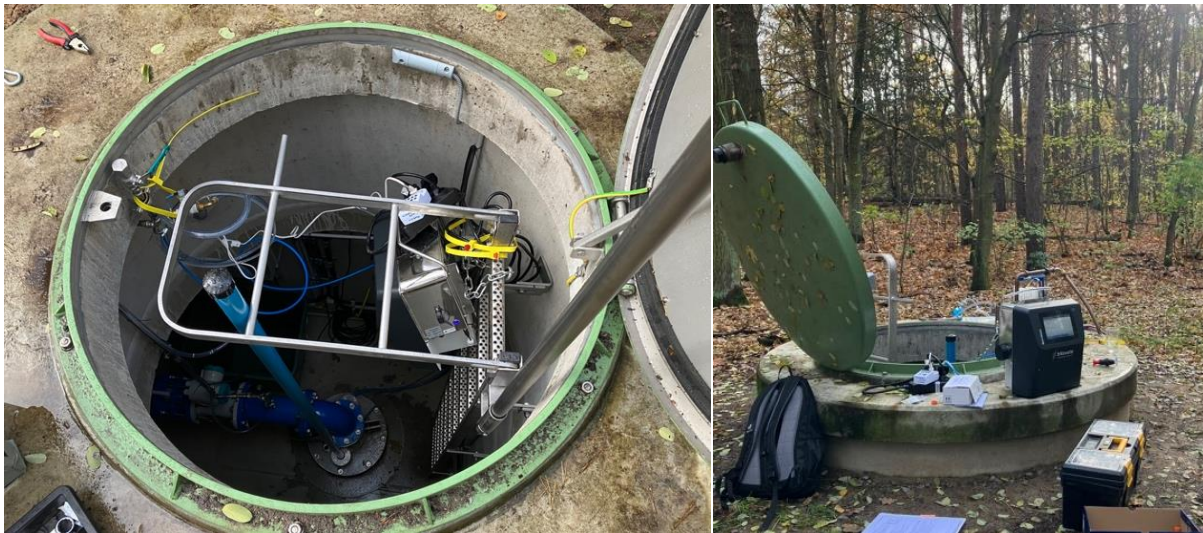
Figure 5: Flow cytometer installed in well chamber (left); flow cytometer maintenance and manual measurements (right)
