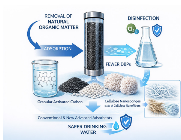
Figure 1 Adsorption of Natural Organic Matter (NOM) to minimize Disinfection By-Products (DBPs) by means of conventional and new advanced adsorbent materials
