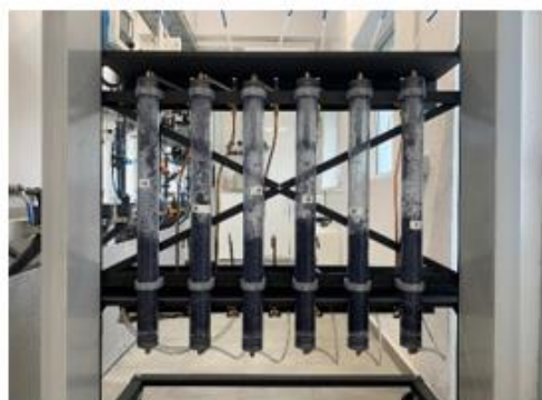
Figure 9: Pilot plant activated carbon columns and description of main operating parameters.
