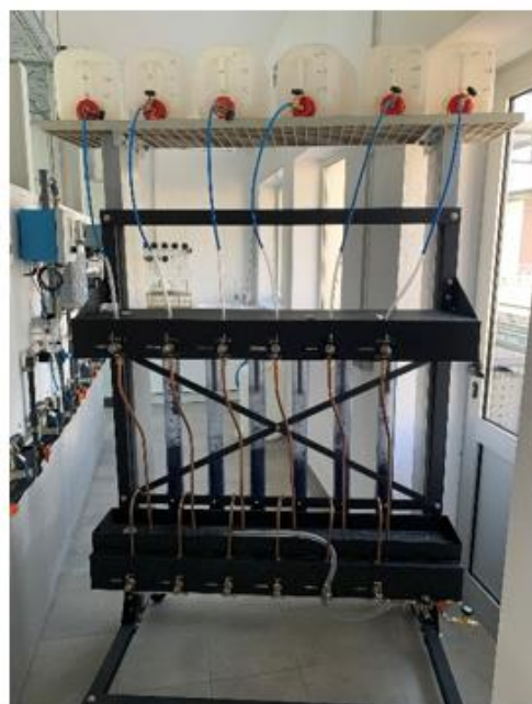
Figure 9: Pilot plant activated carbon columns and description of main operating parameters.
