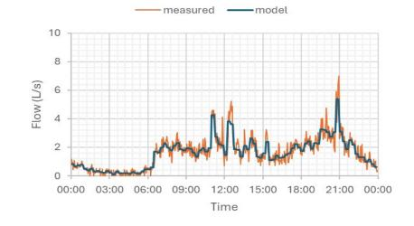
Comparison of flow rate measured and modelled at the exit of Arzila water tank
